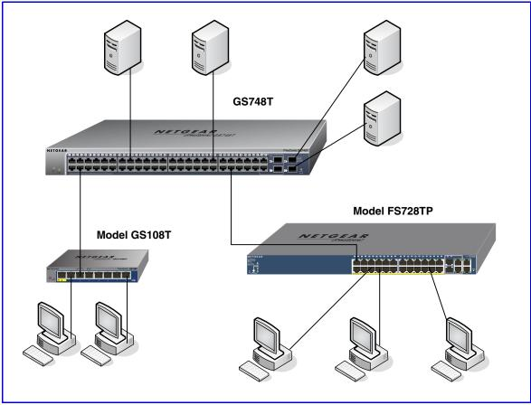
Figure 5. Backbone Switching
